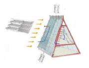
The solutions chosen for the 4 area present a housing system based on triangular residential buildings with double pitched glazed roof directly connected to the ground. One of the two side is completely oriented to the south.
